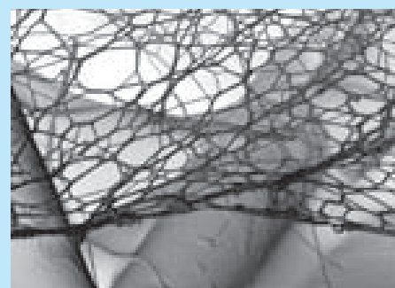
This photo from the scanning electron microscope @ 2500X magnification shows the larger fibers of the substrate under the web of fine fibers.
